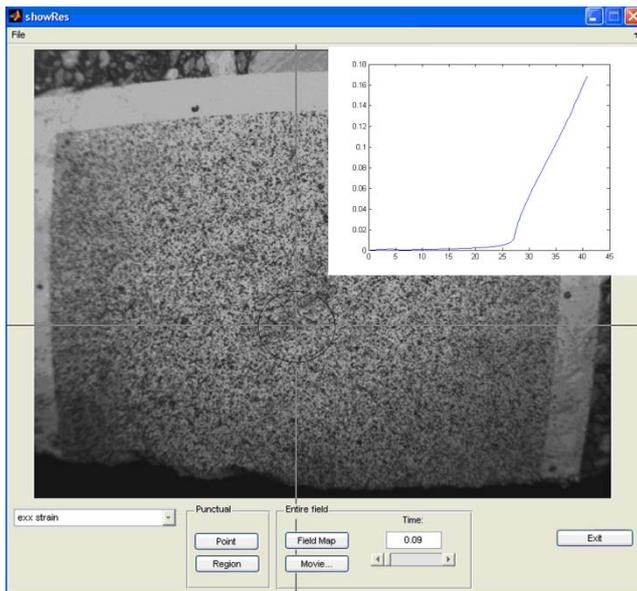
**Figure 3.10** DIC System visual graphic interface
