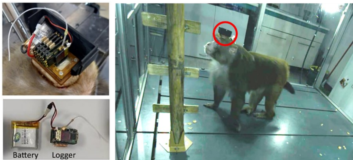
Figure 14 – On the left the recording chamber divided into its components: on the top the open recording chamber; below, the battery connected to the recording system (RatLog-128 by Deuteron Technologies). On the right, the chamber closed with its cover sewn around the components during recording.
