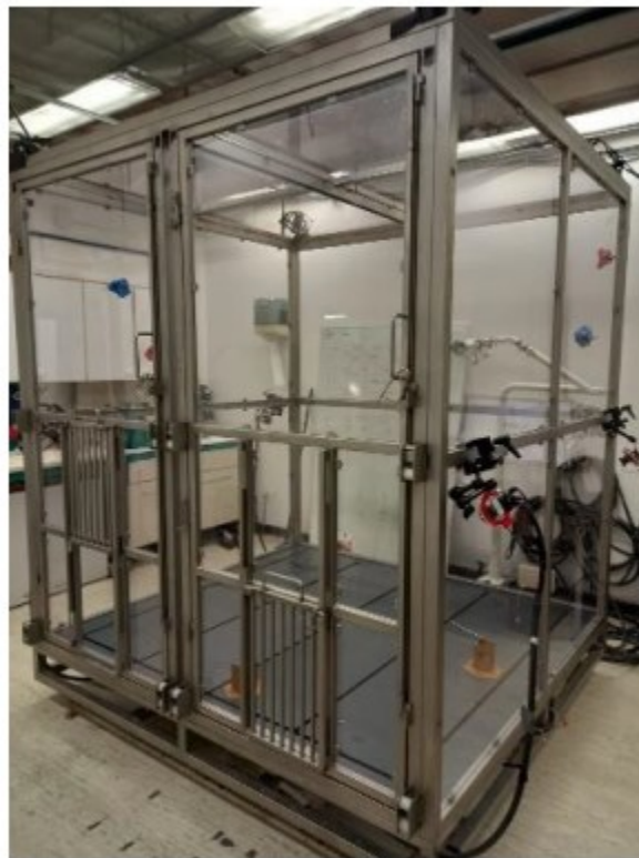
Figure 7. Picture of the NER where all the equipment is visible: the set of 8 cameras, the two large doors with the small opener that allows the monkey to enter, climbing holds, hooks on the roof and on the floor the places where the wooden structure is mounted.
