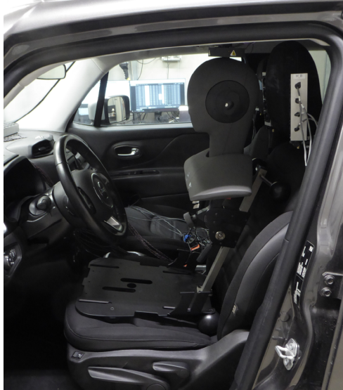
Figure 2.4: DH used for measurements positioned on the driver seat. Courtesy of ASK.
