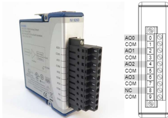
Figure 8 NI-9263 module and corresponding pinouts
