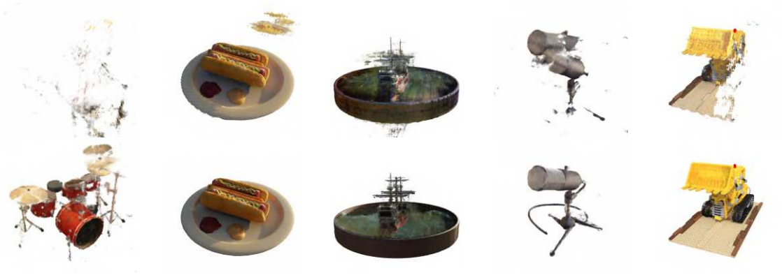
Figure 3.8: Qualitative comparison between choosing poses at random (top row) and using the proposed algorithm (bottom row) in a very few-shot setting ( K = 8 ) [18].
