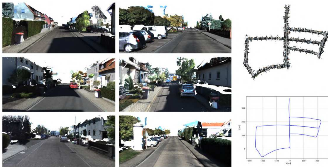
Figure 2.18: 3D reconstruction results from sequence 05 of the KITTI odometry dataset: individual snapshots (left) of the large-scale point cloud (right, top), which is consistent with the estimated camera trajectory (right, bottom).
