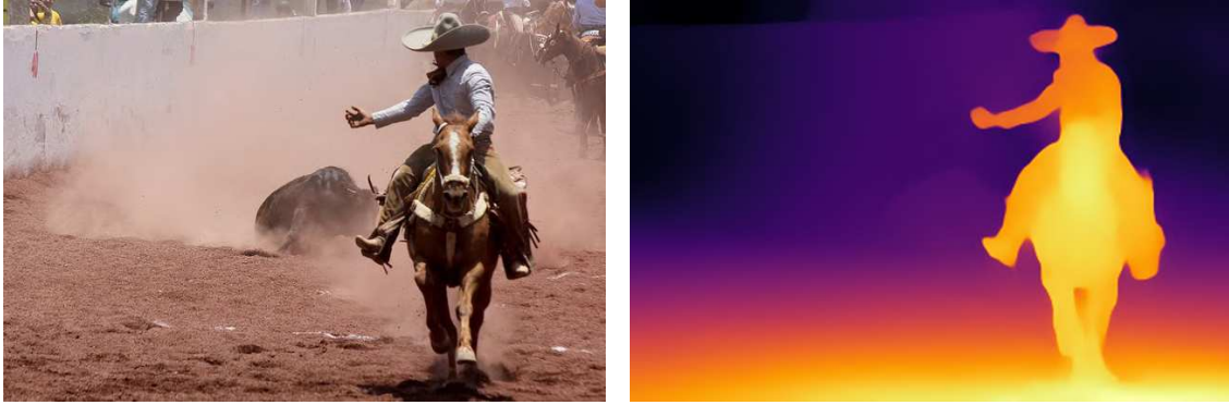
Figure 1.1: Visualization of a depth map computed by a neural network [1]. Darker colors mean farther objects.
