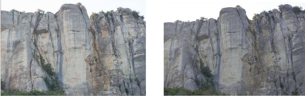
Figure 4-11: Pietra di Bismantova rock wall image pair acquired with the stereo fixed photogrammetric system illustrated in section 4.1.3.
