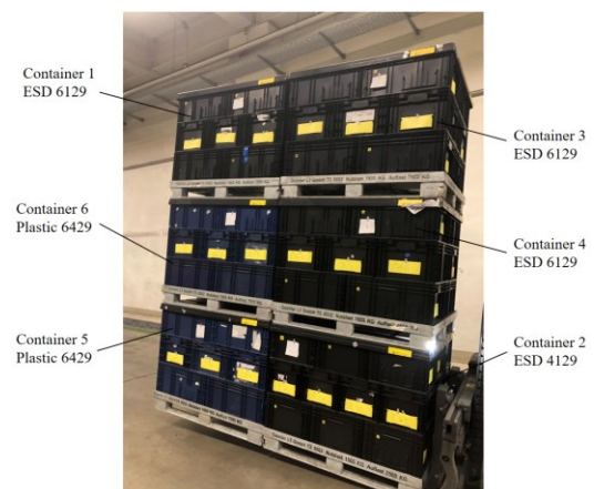
Figure 30 Golden sample for verification of the RFID network planning algorithm
