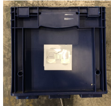
Figure 53 RFID transponder with simulated source of interference (water)
