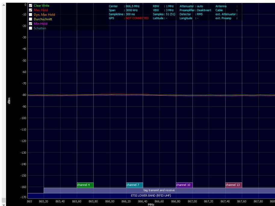
Figure 50 Frequency sweep measurement without simulated source of interference
