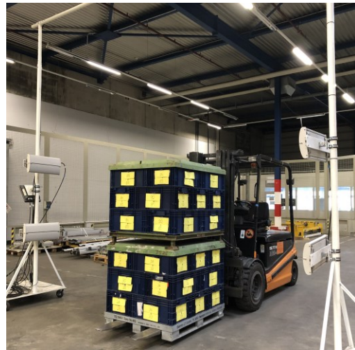
Figure 44 Passage through the RFID gate with the golden sample
