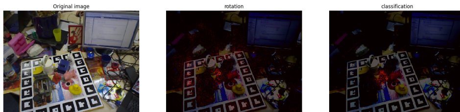
FIGURE 4.7: Vanilla Saliency applied on two images of the Original LineMod dataset. Weights are trained on the same dataset. The gradient is computed given two different outputs: in the second image it is based on the regressor, in the third image it is based on the classifier.
