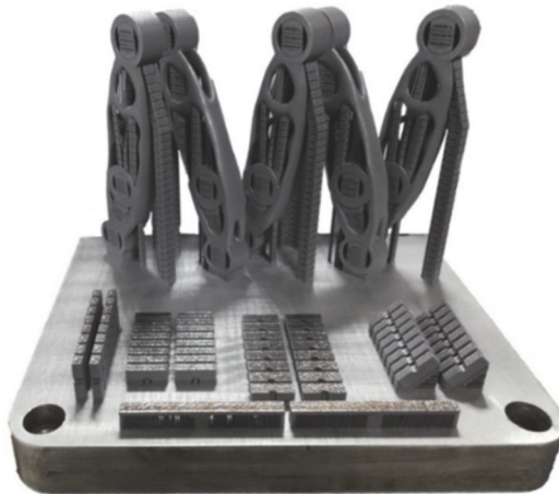
Figure 32 - Build job showing optimized suspension arms, miniature specimens, and software calibration specimens after fabrication and prior to separation from the build platform and support removal
