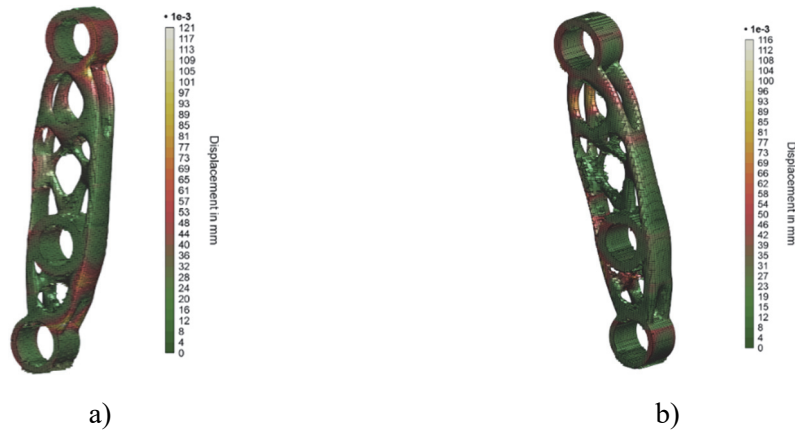
Figure 51 –Displacement of the components after production; a) Orientation A; b) Orientation B
