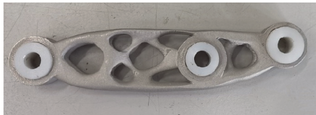
Figure 39 - Optimized component prepared for fatigue testing with nylon bushing positioned inside the part.
