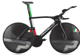
Figure 5 –Pinarello’s Bolide F HR 3D features an additively manufactured Scalmetalloy frame
