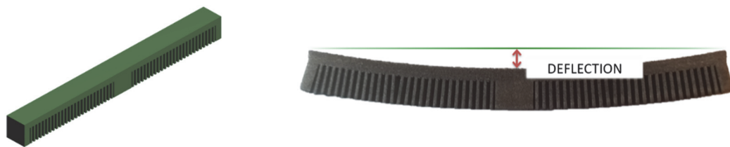
Figure 22 -a) Amphyon process simulation software calibration specimen; b) Method of measuring the deflection of a calibration specimen
