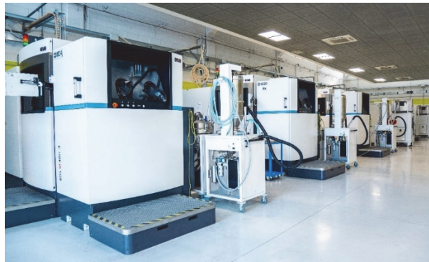
Figure 16 – L-PBF Fabrication systems at the production plant of the company Beamit – Rubbiano (PR) Italy
