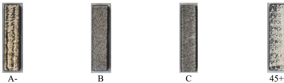
Figure 34 – Flat surface of the miniature samples manufactured alongside the components to characterize the fatigue performance of the material
