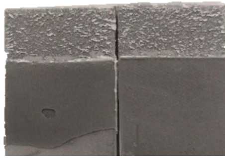
Figure 4-7 – SLJ exhibiting a cohesive type of fracture [179].
