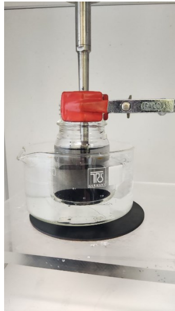
Figure 3-19 – GNPs sonication with Hielscher UP200S-24 kHz high power ultrasonic probe
