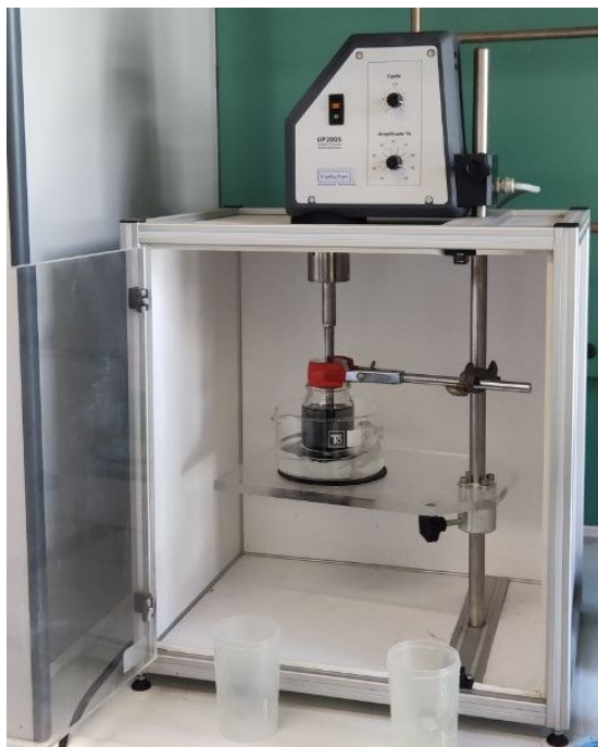
Figure 3-18 – MWCNs sonication with Hielscher UP200S-24 kHz high power ultrasonic probe
