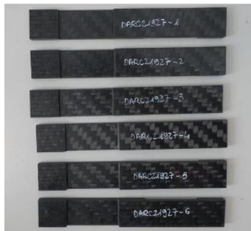
Figure 18 Pristine specimens with PKHP-AcAc 20% for DT120 prepreg.
