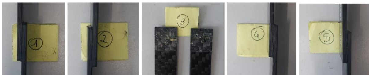
Figure 19 Broken specimens with PKHP-AcAc 20% for DT120 prepreg.
