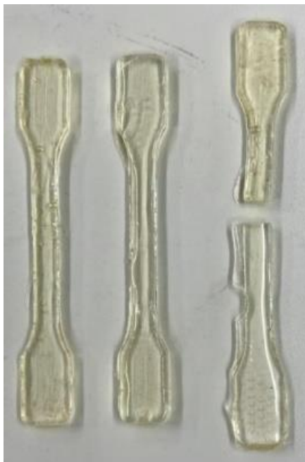
Figure 18 Specimens of polyurethane containing PyPyr-OH : (from left to right) integer, elongated at 2.5 % and broken.
