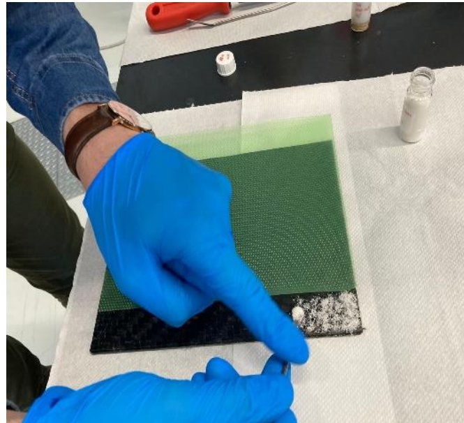
Figure 6 Application of the adhesion promoter in the joint area of prepreg during the preparation of specimens.
