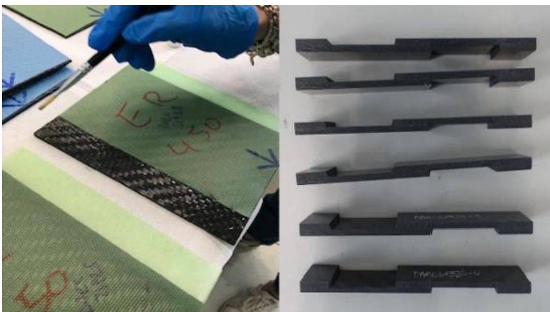
Figure 7 Application of dissolved adhesion promoters in MEK (Left) and the resulting specimens after curing (Right).
