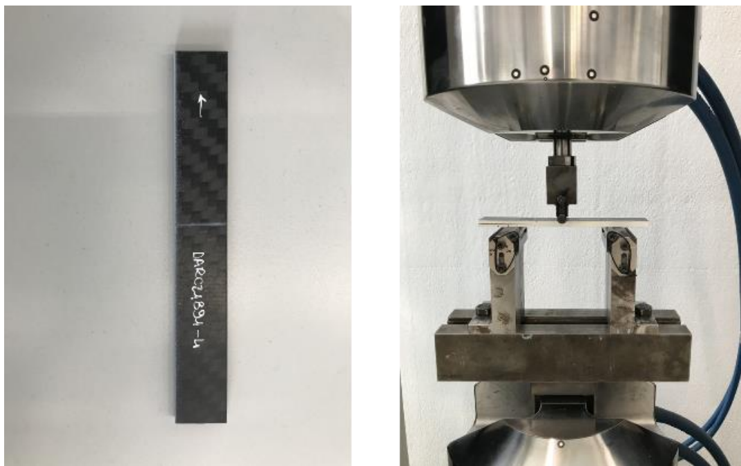
Figure 10 Example of specimen used in fracture toughness test (Left) and the setup for the test (Right).
