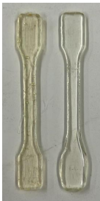
Figure 17 Integer specimens of polyurethane matrix containing PyPyr-OH (left) and PyPyr-OH•CavPOPh (mono -OH) (right).
