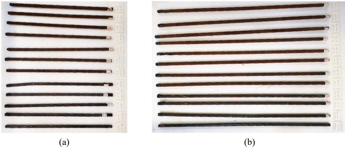
Figure 6-3 Retrieved samples classified as a function of L_i : (a) twelve samples 450 mm long and (b) twelve samples 700 mm long.
