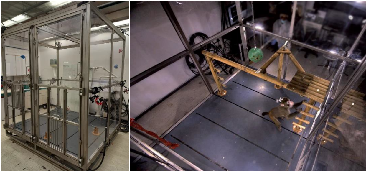
Figure 2.1 – The NeuroEthoRoom (NER), a large Plexiglas enclosure where the sessions are recorded. On the left, a view from the outside, when the enclosure is empty; on the right, a view from the inside, while the monkey is freely moving around the enriched cage.
