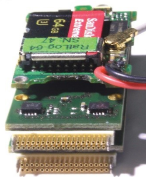
Figure 13 | Deuteron neural logger (RatLog64). RatLog-64 with two stacked headstages
