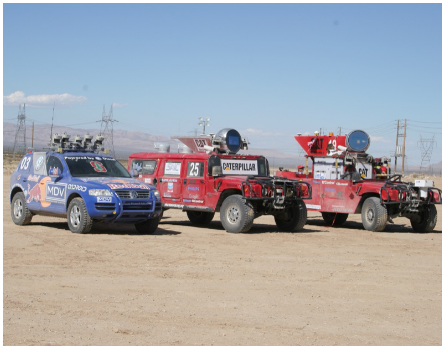
Figure 1.5: Three of the five vehicles that finished Demo II of the DARPA Grand Challenge. On the left the blue vehicle is Stanley, the overall winner from Stanford University's Thrun team. In the center and right, the two red vehicles are Sandstorm and Highlander, which finished second and third, respectively. These two vehicles were developed by Carnegie Mellon University.
