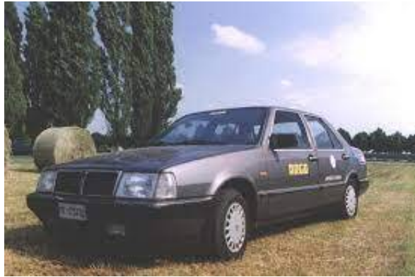
Figure 1.4: The picture represents ARGO, the autonomous vehicle developed in 1998 by Broggi and his team at the University of Parma. A Lancia Thema capable of understanding its surrounding thanks to stereoscopic vision algorithms.
