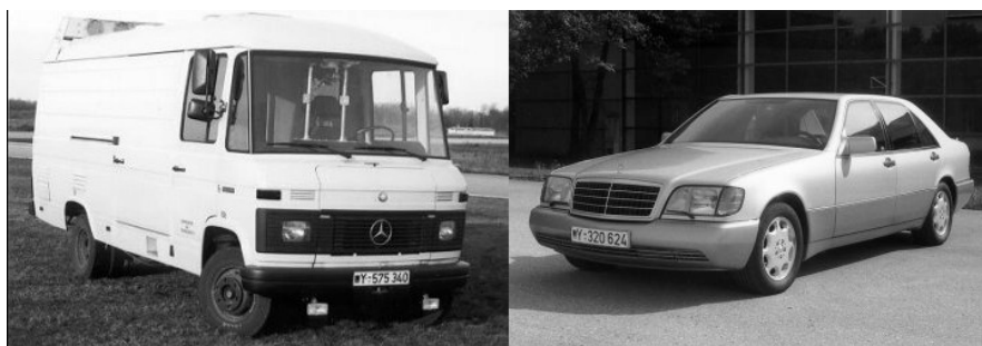
Figure 1.3: The vehicle on the left is VaMoRs, a Mercedes van set up by Dickmanns and his team. It dates back to 1986 and is considered the first autonomous vehicle capable of moving without external auxiliary systems. In contrast, the figure on the right shows Vamp, another autonomous car model developed in 1994 also by the collaboration of Mercedes and Dickmanns.
