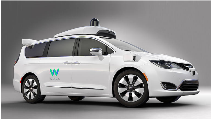
Figure 1.8: The Waymo Robotaxi, with a level 4 automation system.
