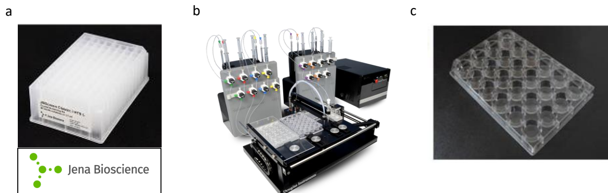
Fig.7: a) commercial crystallization kits with 96 different reservoir solutions; b) robot for automatized hanging drop vapour diffusion screening; c) well plates commonly used to set up manual hanging drop vapour diffusion experiments
