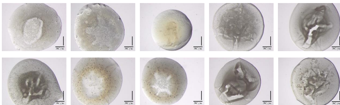
Fig.17: Images obtained by optical microscopy of the heavy precipitant formed during the crystallization between RSL and 2 (top) or 8 (bottom).
