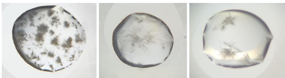
Fig.8: Crystal formation observed during crystallization tests for the RSL- 3 complex performed by a robot sitting drop. The first drop is the control with only compound 3 without protein. The other two drops are
