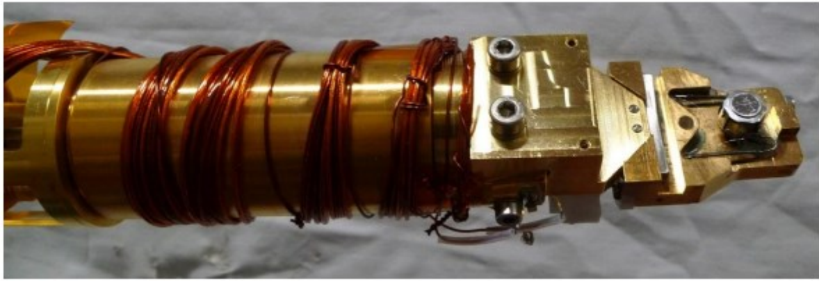
Figure 5 manipulator arm with a sample of Ag(110)
