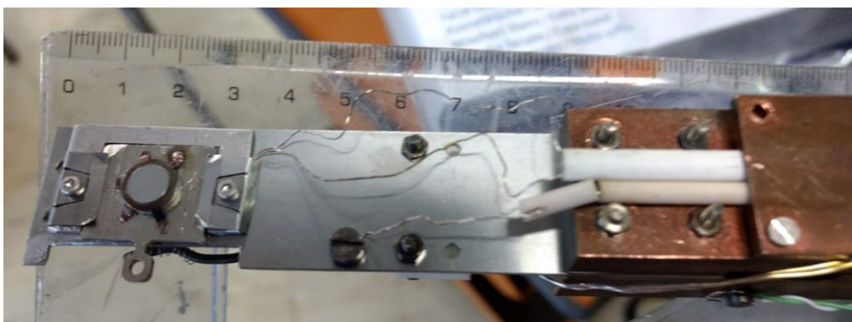
Figure 14. Flag-type sample holder for Omicron instruments. Seen here is a flixed Mo plate with a knob or ring to grab the plate with the sample on top. The electrical connections (bias voltage, thermocouple) is attached to the receptacle where the sample holder is held by tabs on either side. This is designed for easy sample transfer without breaking the vacuum (using an FEL).
