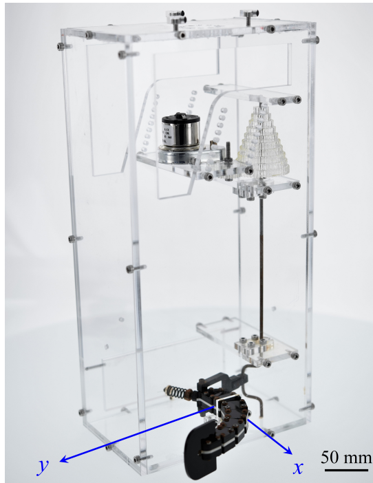
Figure 9.4. Detail of the driving system, mounted onto the load cell: the motor is connected through gears to a crankshaft and the snapping beam is actuated by a crank.
