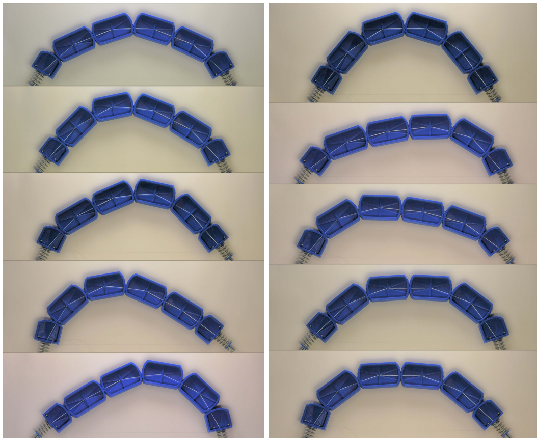
Figure 5.18. Experiments on the prototype of the bi-stable flex-ten beam considered in Figure 5.6 ( n = 6 , Prototype A ). The ten inhomogeneous equilibrium configuration in the hard device for \Delta\bar{\varphi} = 120.00^\circ = 2.0944 rad.
