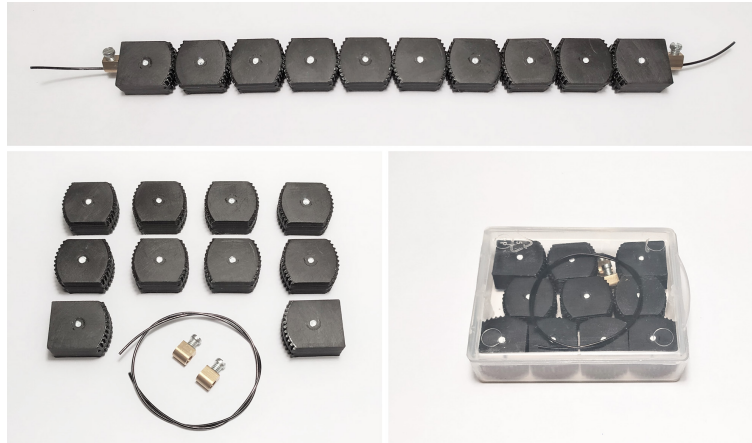
Figure 1.5. Packaging of a flex-ten assembly: beam in the deployed straight state, disassembled beam (segments, cable and clamps to anchor the cable) and components packed in a prismatic box for transportation.
