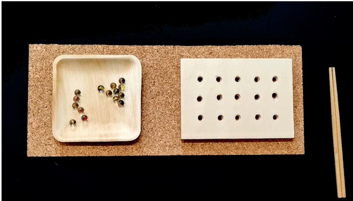
Figure 3.1 Kit adopted for the motor task. The kit adopted for the motor task was composed of a squared plane bowl (size 15.2 x 15.2 x 1.5 cm) and a rectangular wood board (20.4 x 14.5 x 1.5 cm) with fifteen holes distantiated by 7.2 cm. The holes' diameter is 1.1 cm (1 mm lower than the diameter of the marbles). Each hole was distantiated from the closest one by 2.5 cm. The length of the wood chopsticks is 24 cm.
