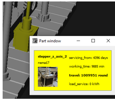
Figure 2.31: The image shows one of the Z-axis motors in a REQUIRE ACTION state for exceeding the maximum number of rotations.
