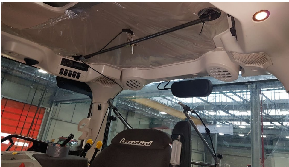
Figure 3.39: Microphone in the center above the head
