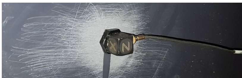
Figure 3.5: Accelerometer glued to the structure
