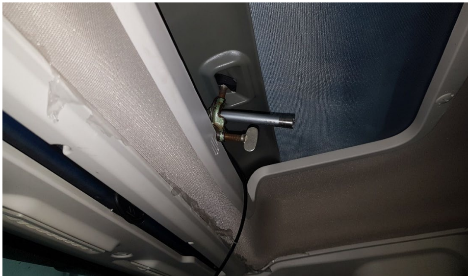
Figure 3.38: Front microphone near the Bluetooth speakerphone
