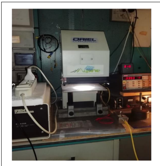
Fig.2.10 Photograph of the Oriel solar simulator used to test the effective solar blindness of photodetector.
