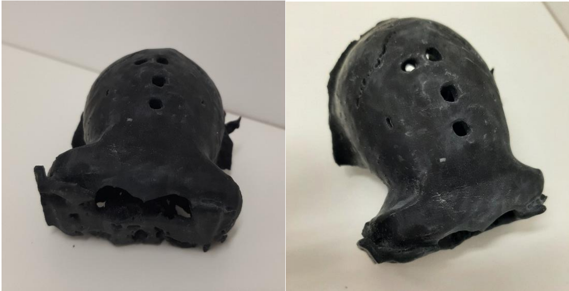
Figure 17. Example of 3D print of the skull. 1:1 model of the Mk2 skull. The holes specify stereotaxic coordinates of interest to be considered for the positioning of the headpost and, subsequently, of the recording probes.
