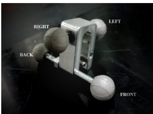
Figure 7. Image of the custom-made structure with the four retroreflective markers which is attached to the monkey’s head-post in the NER condition in order to extract the 3D position of the animal.
