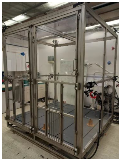
Figure 3. The NeuroEthoRoom. The picture illustrates a view from the outside of the large plexiglass enclosure where the sessions are recorded.
