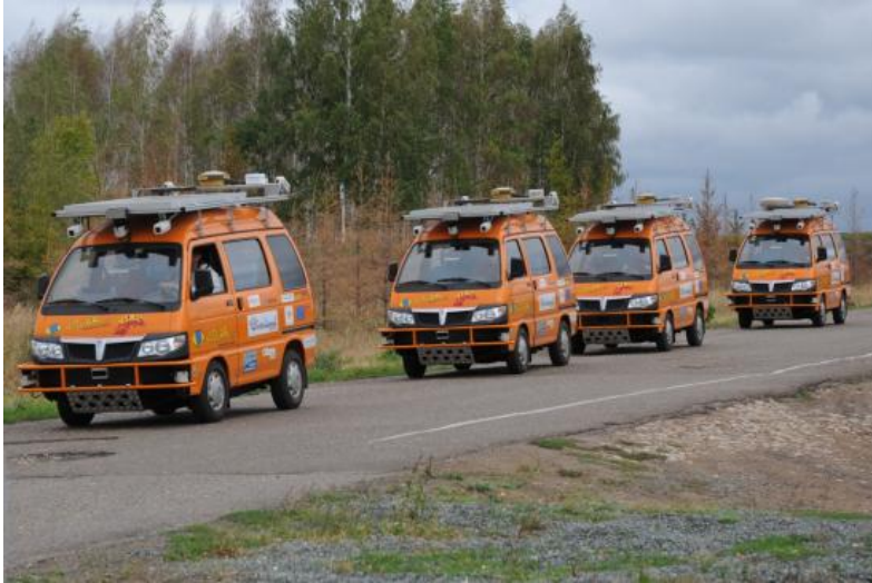
Figure 6: The four self-driving Piaggio Porters developed by VisLab which travelled from Parma to Shanghai
