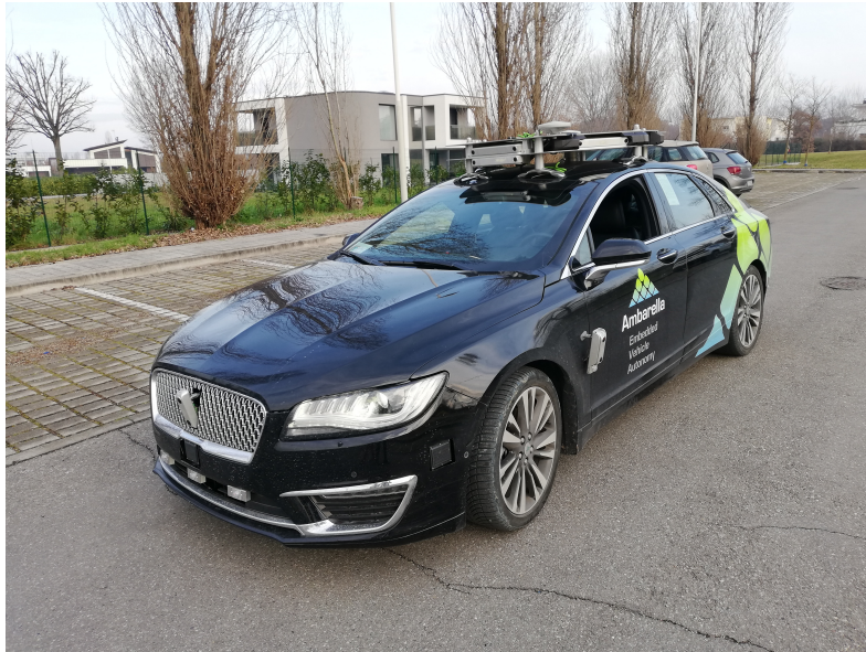
Figure 4.12: The real autonomous driving car used to perform tests on the real roundabout of Figure 4.7g.
