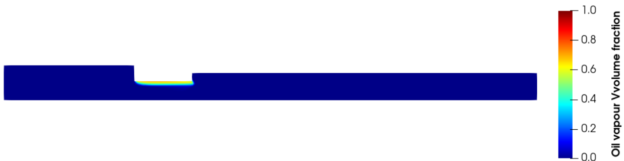
Figure 4.37. Vapour volume fraction distribution through the orifice. Pressure drop 0.43 bar, Set A of parameters.
