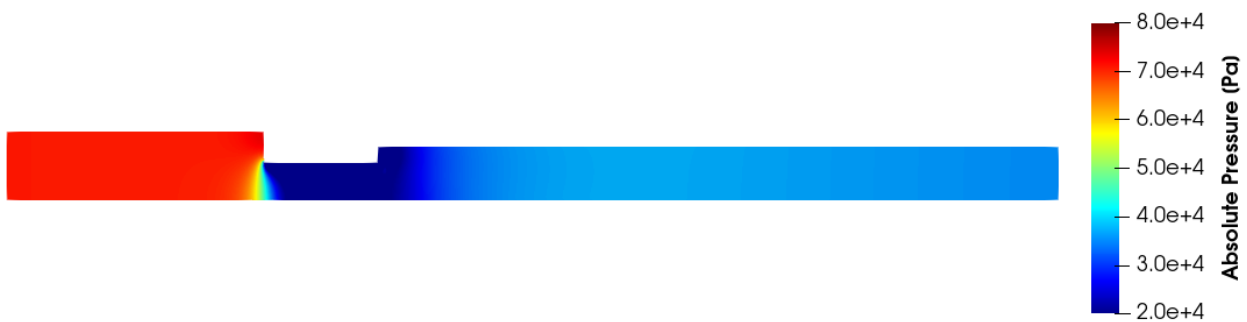
Figure 4.35. Pressure distribution through the orifice. Pressure drop 0.43 bar, Set A of parameters.
