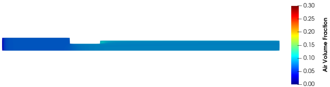
Figure 4.34. Air volume fraction distribution through the orifice. Pressure drop 0.256 bar. Set A of parameters.
