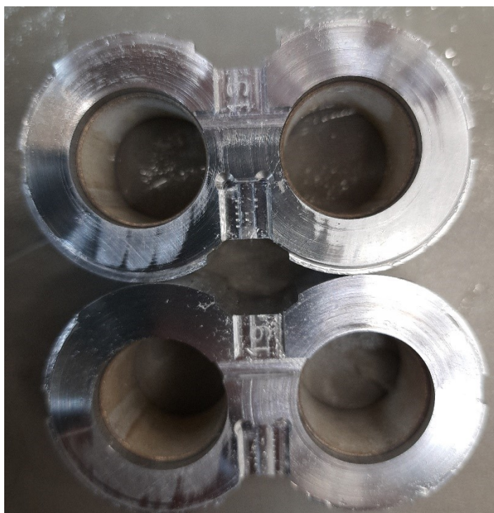
Figure 6.48. Photos of the lateral plates of the baseline pump 1 after Cycle I and Cycle II
