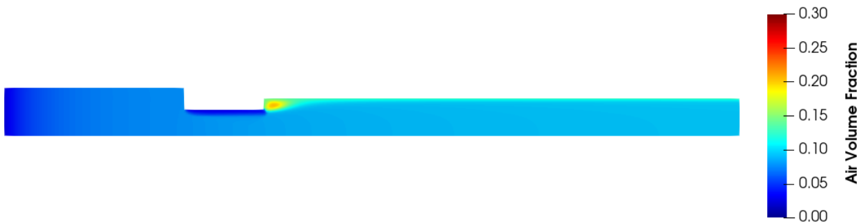
Figure 4.36. Air volume fraction distribution through the orifice. Pressure drop 0.43 bar. Set A of parameters.
