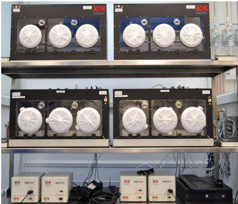
Figure 6. Ad hoc incubators developed by Okolab
