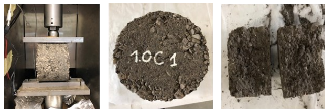
Figure 12 – Indirect tension test specimen and configuration
