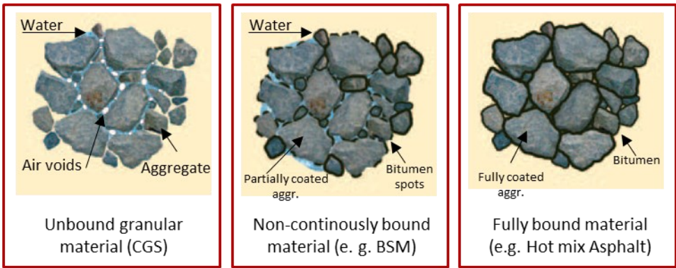
Figure 4 - Unbound, partially bound and fully bound pavement material scheme, adapted from Wirtgen (2012)
