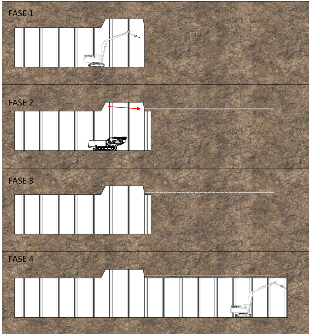
Figure 4.5 Phase 1: Tunnel excavation until the monitored section and pilot tunnel realization; Phase 2: Horizontal borehole; Phase 3: Pre-Conv Array installation; Phase 4: Tunnel advance and monitoring of induced deformations. Figure adapted from (Savi et al., 2019)
