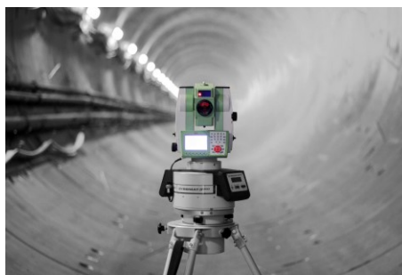
Figure 3.9 Example of a geodetic survey in tunnels (source: Monteith & Sutherland survey)
