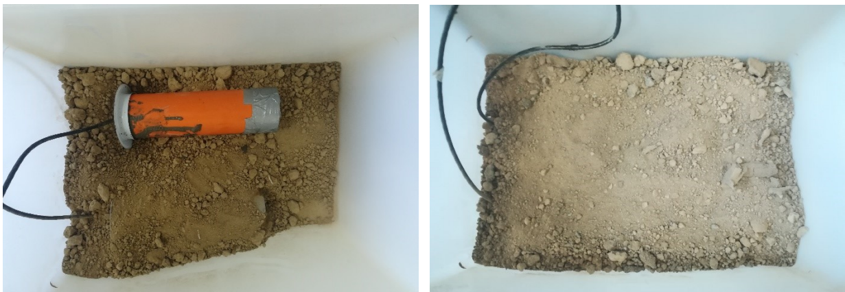
Figure 5.8 Sensor placed inside plastic box and surrounded by ground
