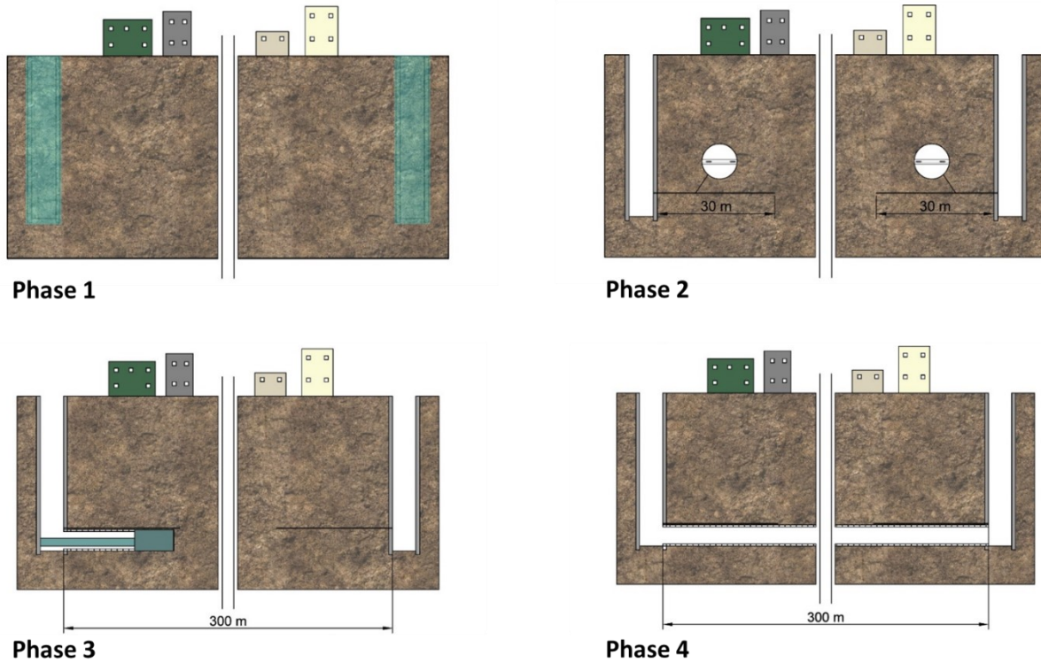
Figure 4.9 Phase 1: The TBM excavation is preceded by two vertical shafts excavation for TBM positioning and retrieval; Phase 2: Two horizontal boreholes above tunnel crown are realized to insert the Pre-Conv Array; Phase 3: TBM excavation and monitoring of vertical displacements; Phase 4: Monitoring of vertical displacements during tunnel operational phase. Figure adapted from (Savi et al., 2019)
