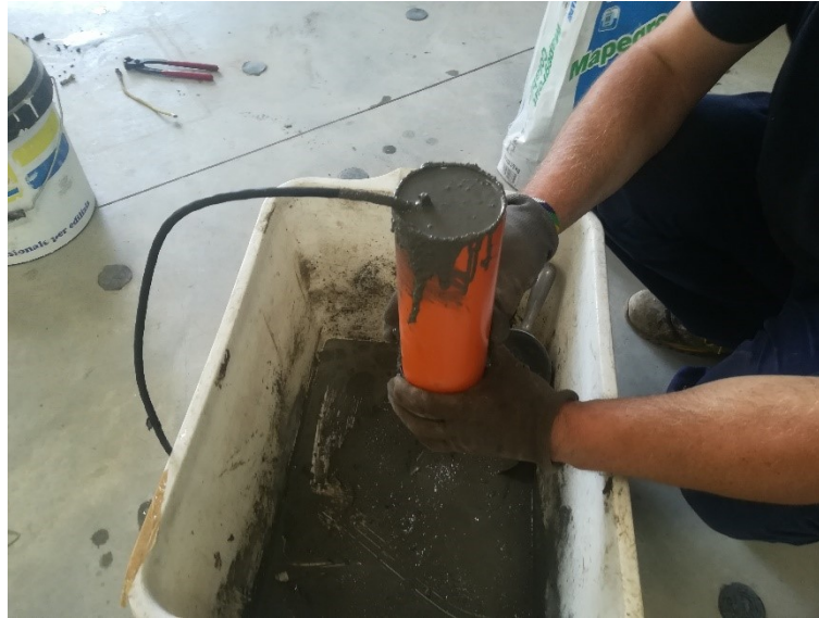
Figure 5.7 Sensor immersed in the concrete mortar inside a PVC casing
