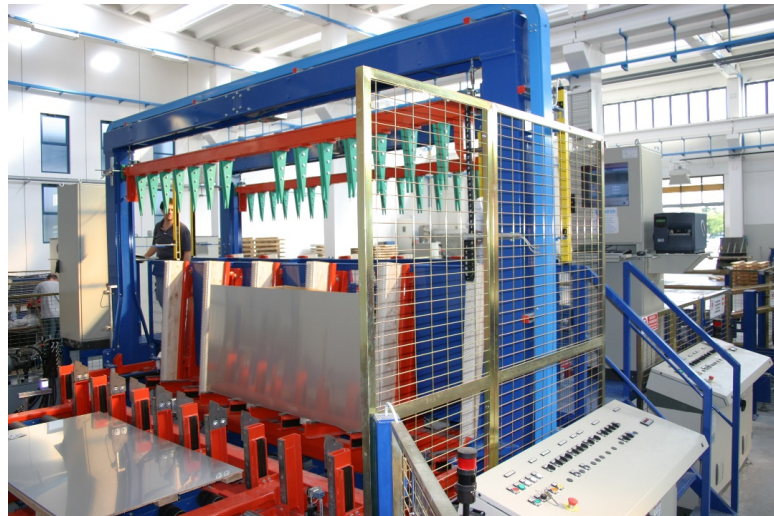
Figure 2.4. Machine for picking in metal sheet AS/RS.
