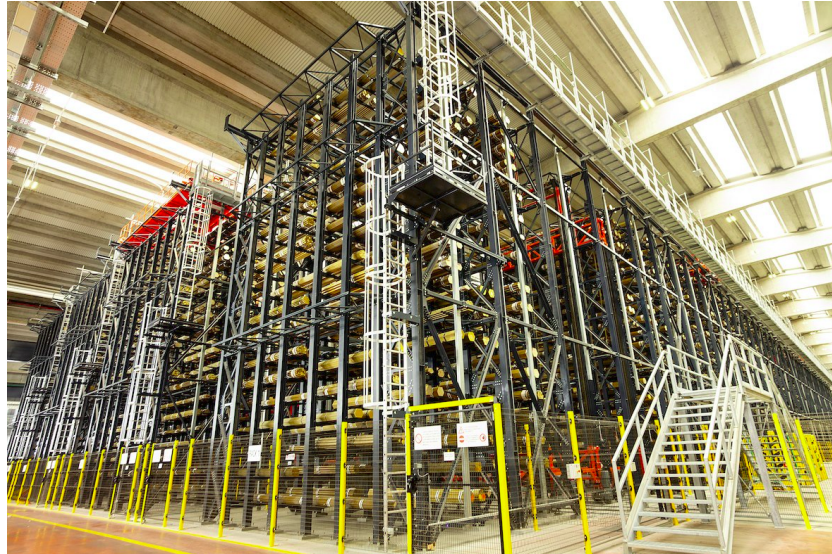
Figure 2.6. Picture of a Shuttle-Lift-Crane AS/RS [4].
