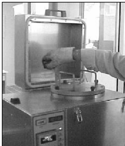
Figura 5-4: Pressure Aging Vessel (PAV)
