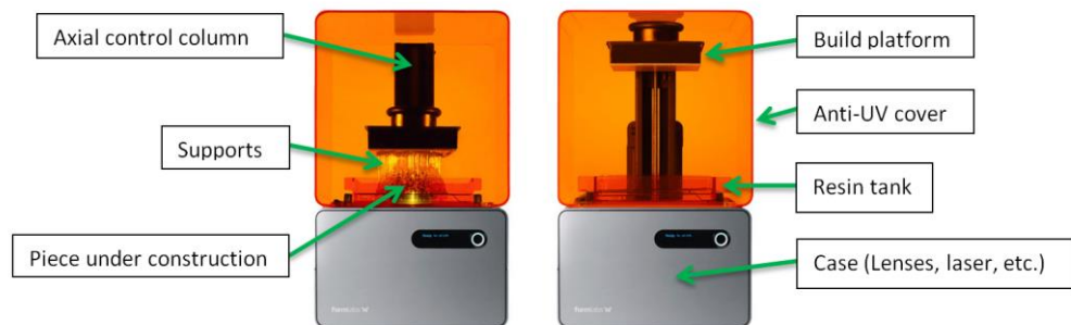
Figure 27: Form 1+ components scheme
