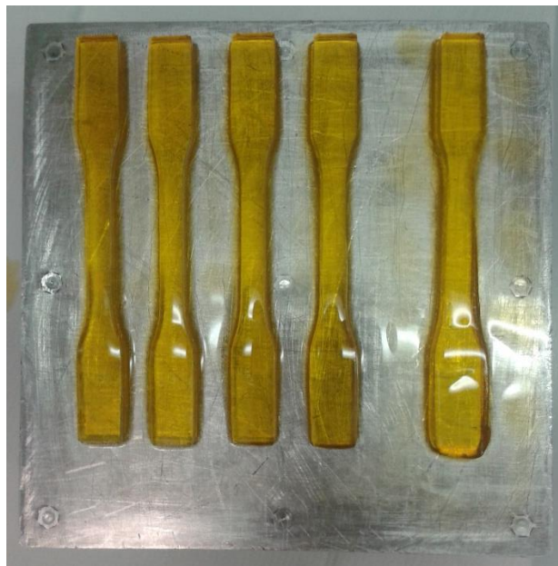
Figure 38: better sample disposition results, the sample on the right is still somehow slightly overcured
