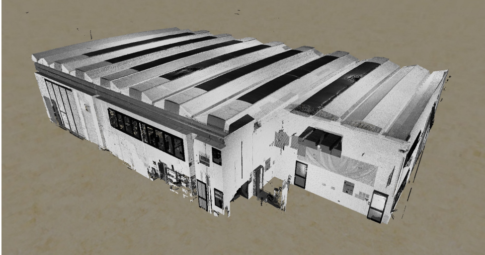
Figure 6.15: Point cloud from survey performed with Leica Scanstation P30 using the optimized scan stations ( \theta_{min}=35^\circ ).
