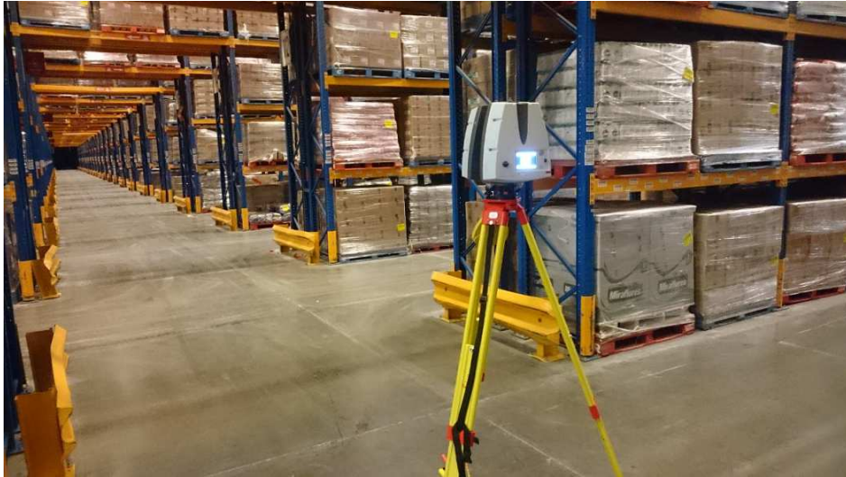
Figure 1.5: Terrestrial Laser Scanning survey in a warehouse using a Leica ScanStation P30 mounted on a tripod.
