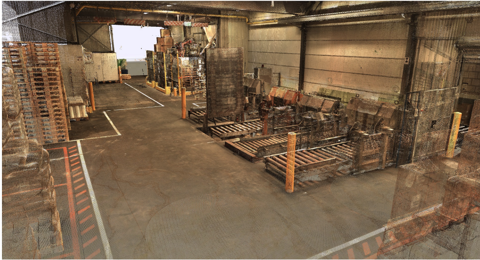
Figure 1.1: Example of point cloud acquired with a Terrestrial Laser Scanner.
