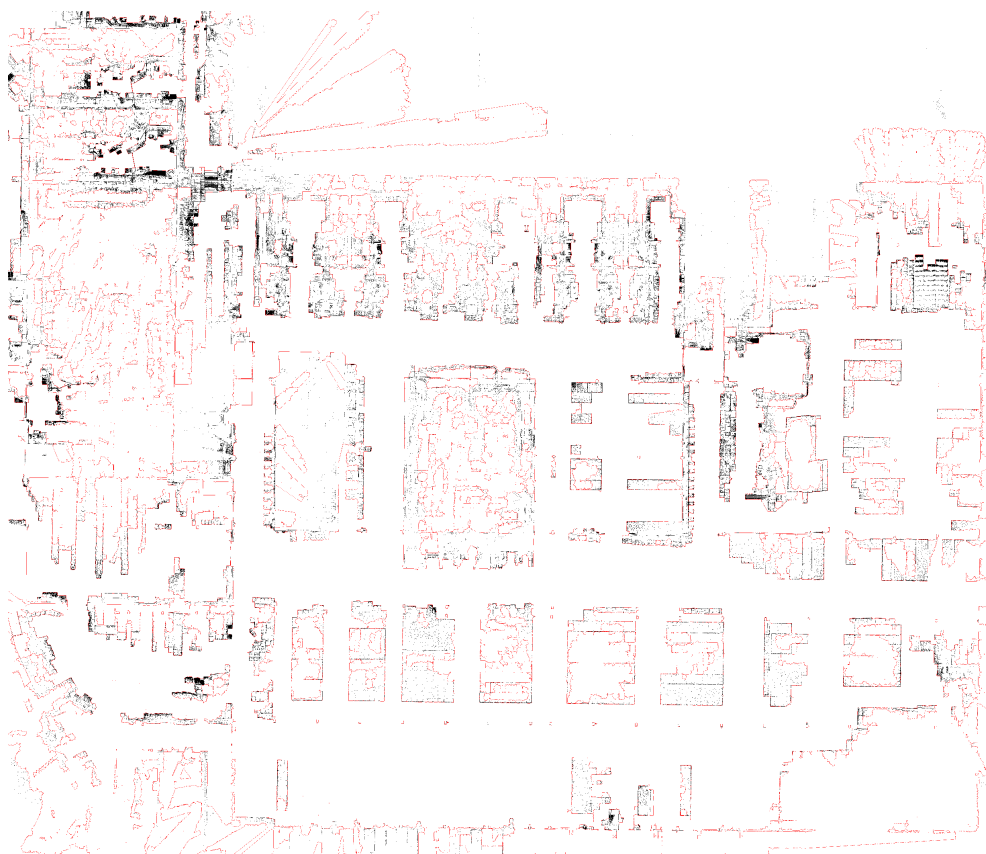
Figure 4.11: Floor plan of Dataset06 with r_v = 5 cm. Black dots are points in A^+ (Section 4.2.4). Some artifacts are visible in non-critical regions where few scans were performed or outside the perimeter walls..
