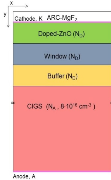
Figure 5.25: Schematic cross-section of the structures with Zn_{1-x}Mg_xO window interlayer and Zn(O,S) buffer.
