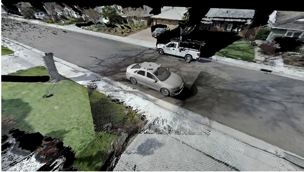
Figure 1: Full 360° 3D reconstruction based on the perception of a complete set of stereo cameras.
