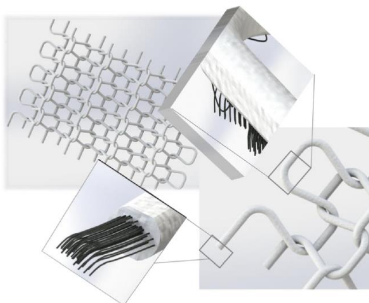
Figure 6.48: Hypothetical model of a conductive cardiac patch: SiC NWs (in black) are present inside the Teflon wires (in white).
