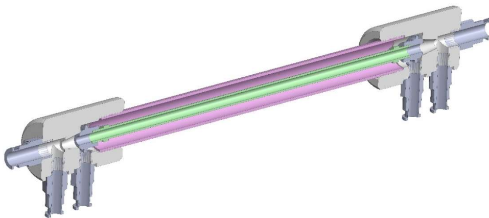
Figure 6.6: 3D CAD model of the here developed shell and tube heat exchanger
