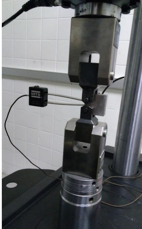
Figure 13 - shows the experimental apparatus for fracture test with a C(T) specimen.
