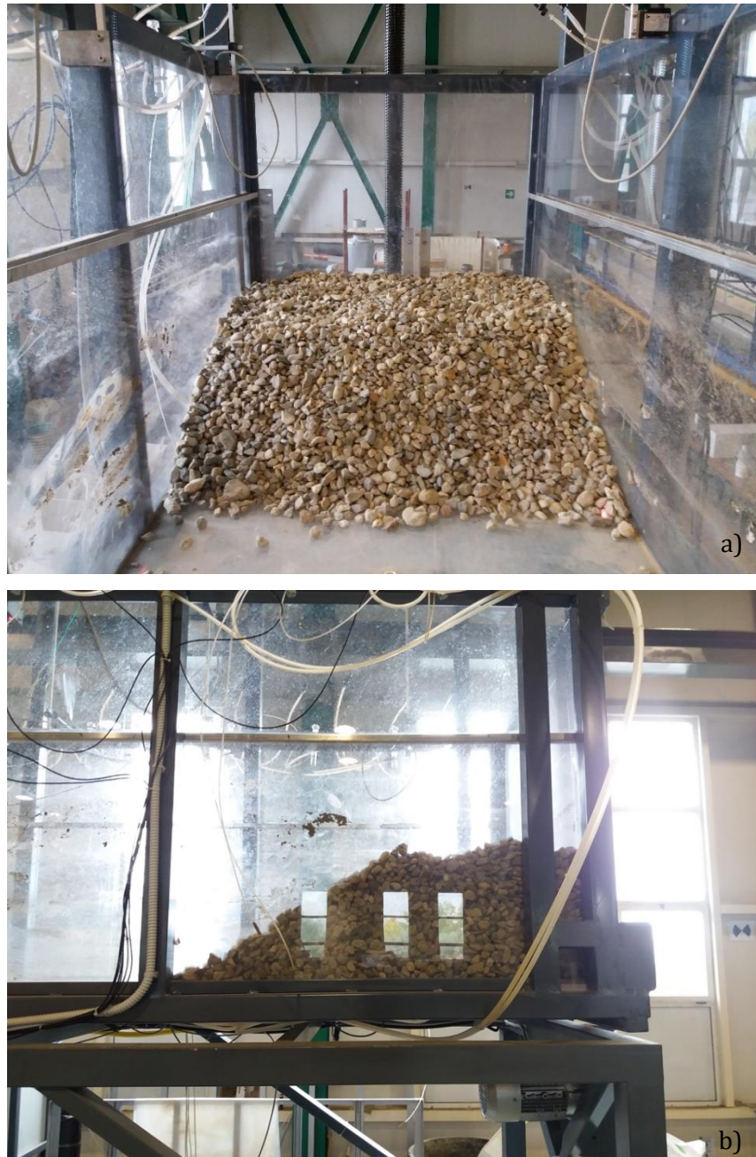
Figure 6.21: Granular material simulating debris flow; a) Front view; b) Lateral view
