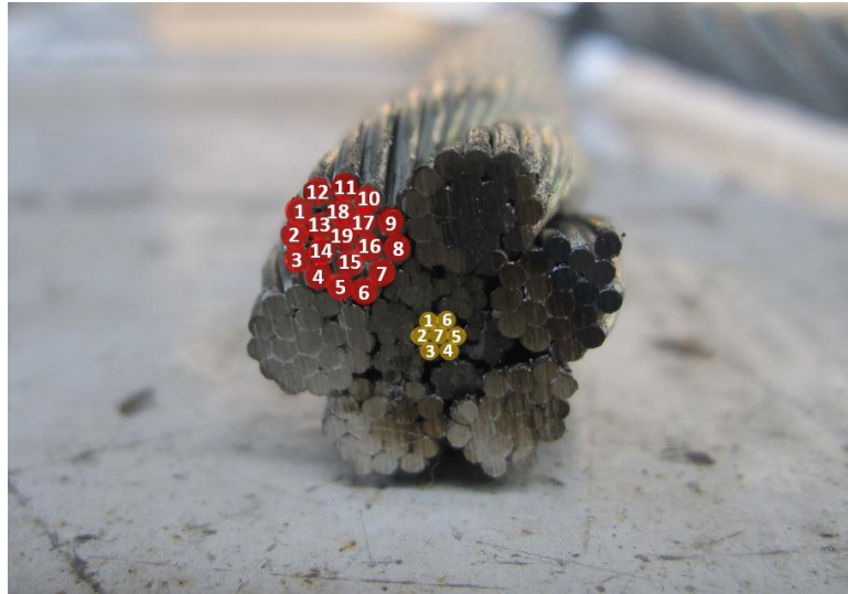
Figure 4.46: Wire rope 12 mm section – number of wires and detail
