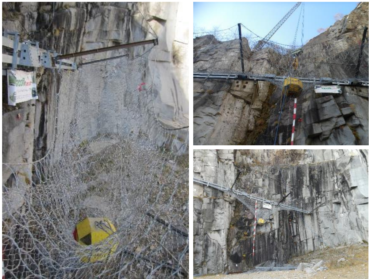
Figure 5.39: Block stopped by the barrier; a) Lateral vie; b) Bottom view and c) Overall system at the end of the test
