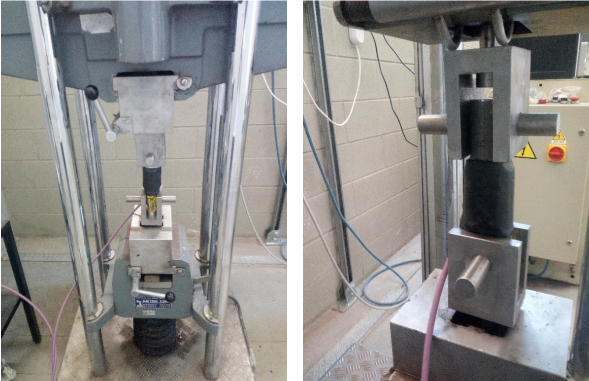
Figure 7.14: Laboratory test on load cell; a) Traction test configuration and b) load cell with circuit protection cover
