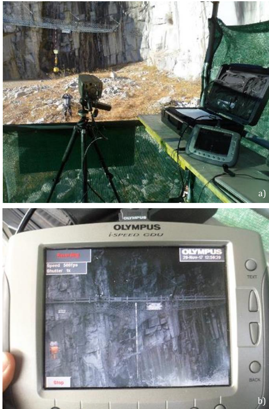
Figure 5.11: High-speed camera; a) Location in the test area and b) Recording process
