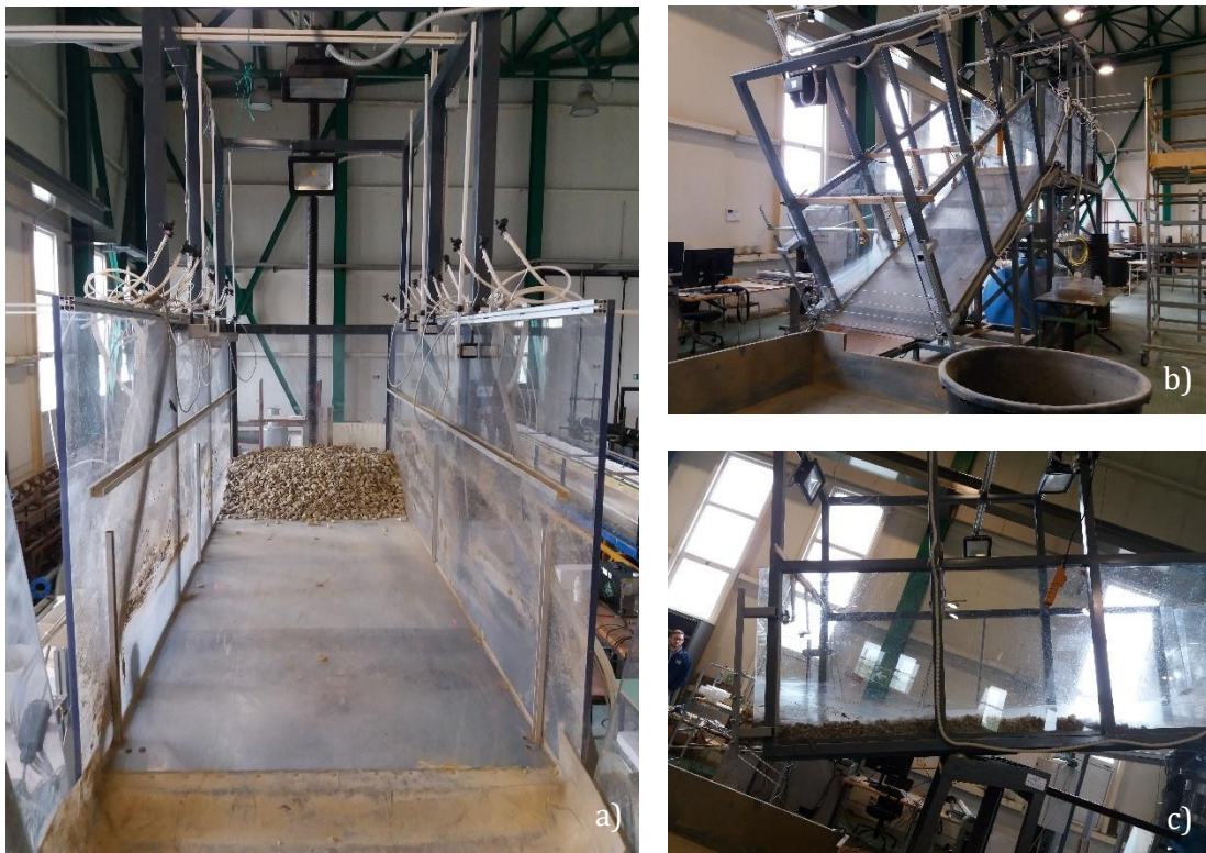
Figure 6.19: Photos of channel used for debris flow laboratory test at the University of Cosenza (CAMILab); a) Front view of the channel bottom and granular material preparation; b) Test configuration with change of the inclination of the downstream part of the channel; c) Channel lateral view with some granular material accumulated behind the barrier after the test
