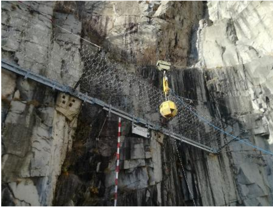
Figure 5.12: SEL block and release mechanism
