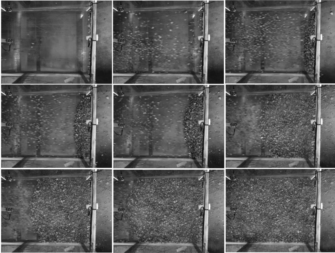
Figure 6.30: Images of the impact phase recorded during experiment n. 3 and elaborated through the dedicated PIV software
