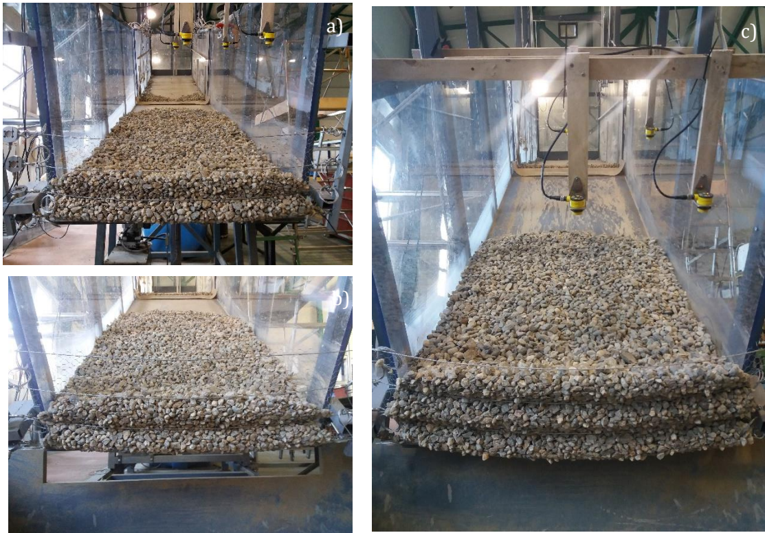
Figure 6.23: Material accumulated behind the barrier at the end of the experiments; a) Case 1 with channel inclination 30^\circ and 4 longitudinal ropes; b) Case 2 with channel inclination 33.25^\circ and 4 longitudinal ropes; c) Case 3 with channel inclination 36.5^\circ and 4 longitudinal ropes
