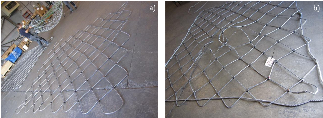
Figure 4.25: Tested HCP panel; a) Specimen before test and b) Specimen brake due to loading process
