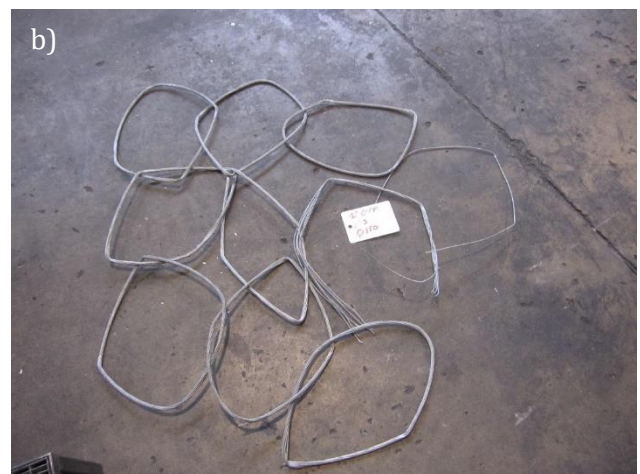
Figure 4.40: Tested ring panel; a) Specimen before test and b) Specimen brake due to loading process
