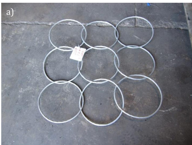
Figure 4.40: Tested ring panel; a) Specimen before test and b) Specimen brake due to loading process
