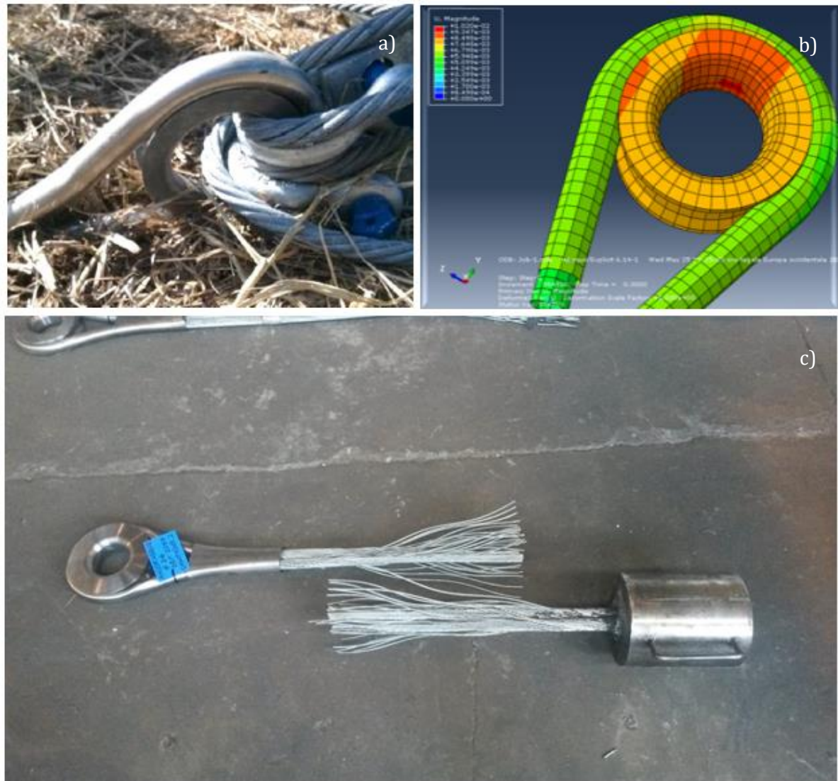
Figure 4.57: Flexible anchorage system; a) Application on site; b) Numerical model of the anchor head and c) Tested anchor with broken rope
