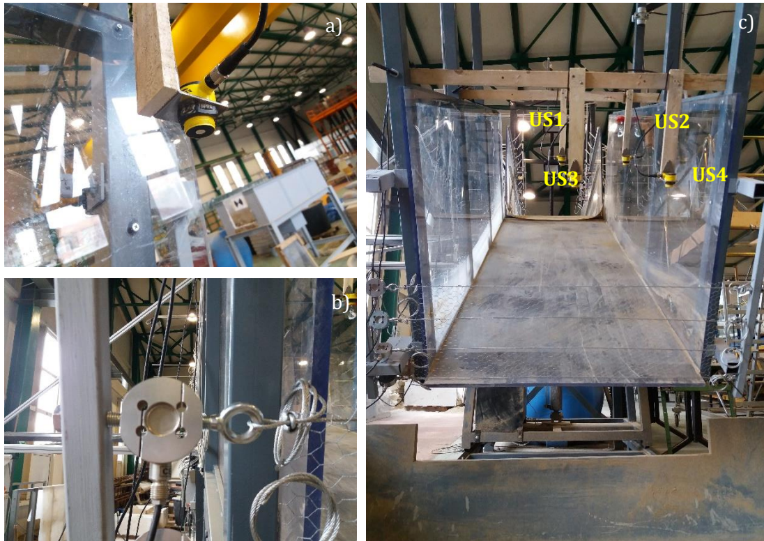
Figure 6.20: Photos of measurement devices used for laboratory flume test; a) Ultrasonic level device for measurement of the flow height; b) Load cell connecting barrier and rigid structure for measurement of rope tension; c) Instrumented channel and devices numeration
