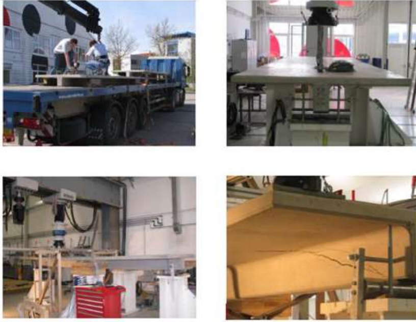
Figure 13. Test of T-shaped prestressed concrete girder
