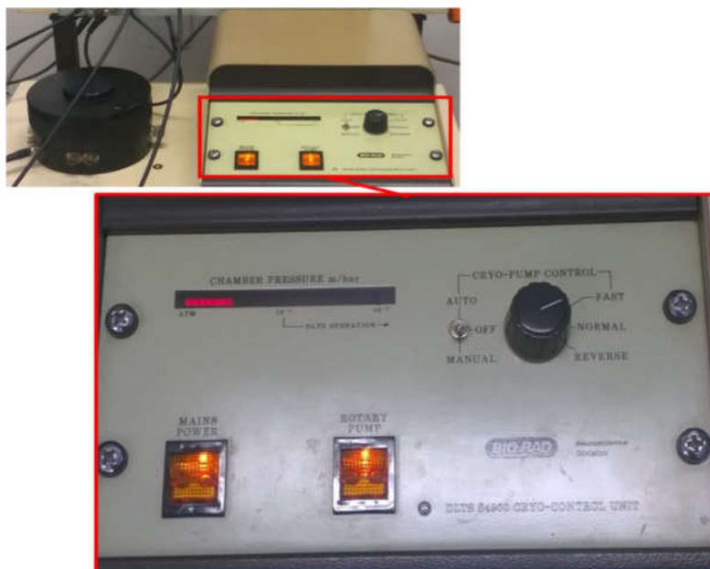
Figure 29 BIO-RAD control unit used to monitor the pressure inside the cryo-chamber and regulate the rotation speed of the rotary pump, which was used to control the liquid nitrogen flow into the cryostat. During temperature dependent measurements, , settings 'Auto' and 'Fast' were used for the cryo-pump.
