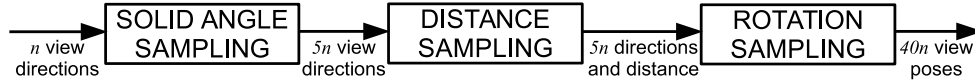
Figure 3.2: Flowchart of viewpoint generation (line 2 in Algorithm 4). Each candidate view direction generates 40 view poses for the sensor.
