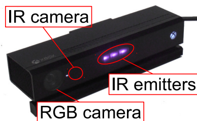
Figure 3.11: The Kinect V2 sensor with IR camera, RGB camera and IR emitters.
