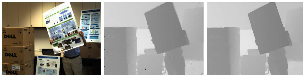
Figure 1.5: RGB image (left), noisy depth image (center) and enhanced depth image using temporal mode filter (right). Image source: [5] © 2012 IEEE.
