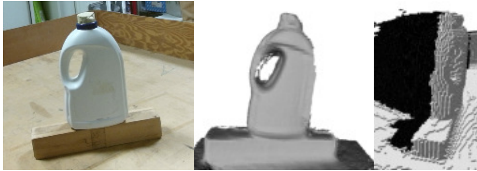
Figure 3.5: Left: a jug observed from the current sensor viewpoint. Center: the 3D mesh reconstructed by KinFu. Right: the volumetric representation (rotated view), with occupied (white) and unknown (black) voxels.
