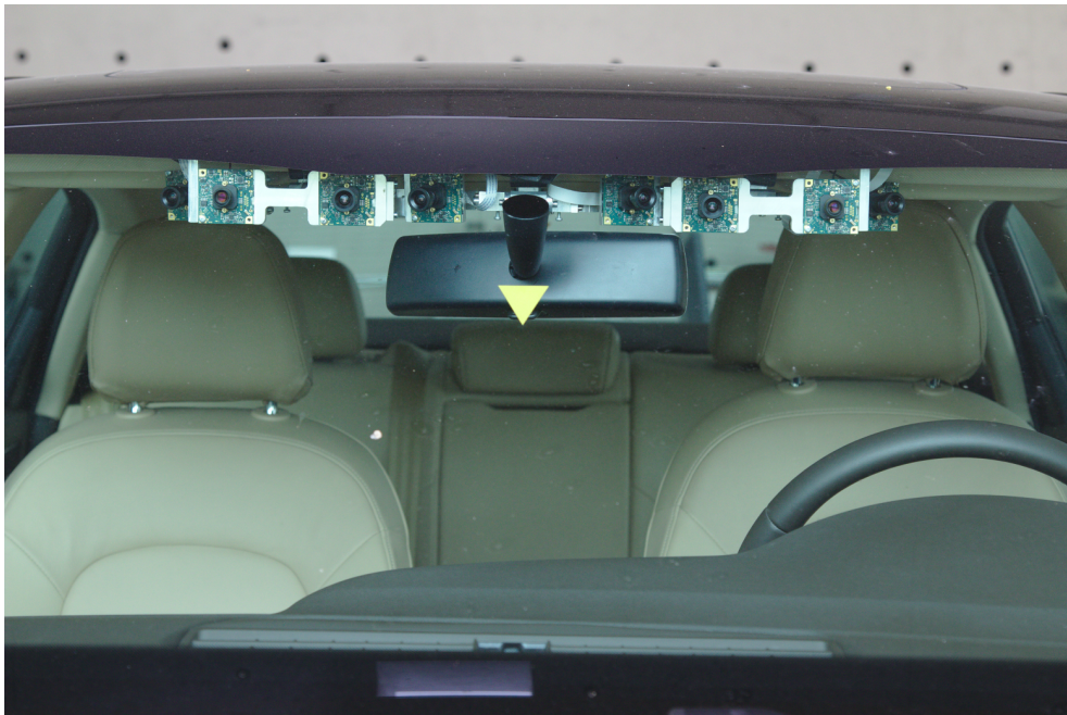
Figure 1.10: The frontal camera rack. It provides medium and far range image coverage.
