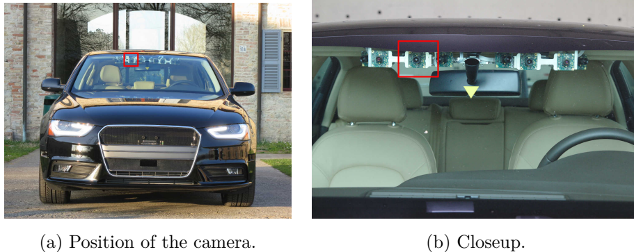
Figure 2.7: The right camera of the FFN stereo couple is used to acquire the images in the dataset.
