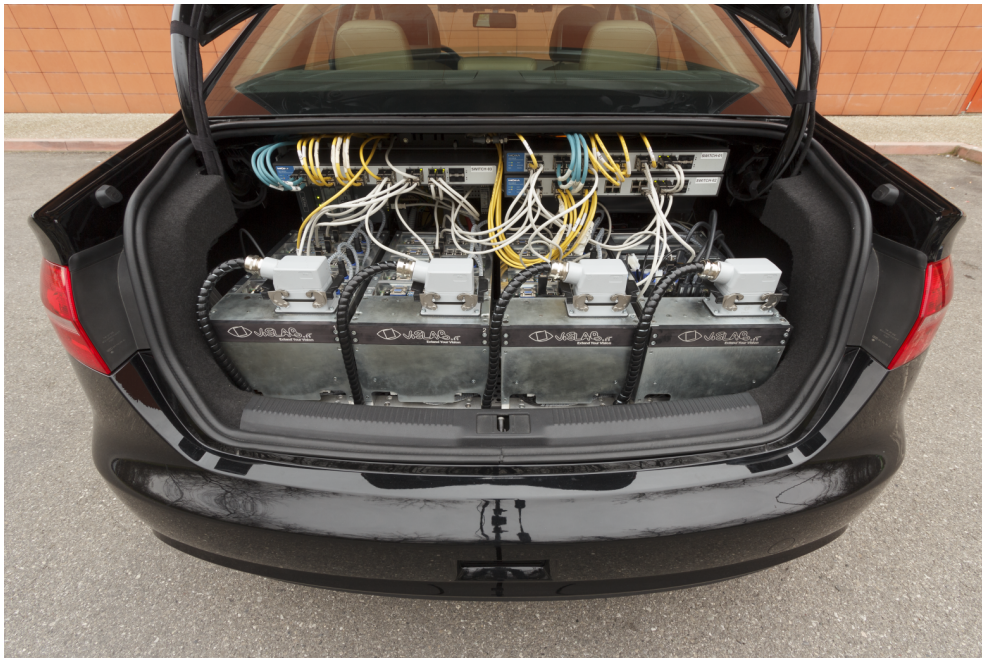
Figure 1.12: DEEVA's computing hardware: up to 20 PC connected with 3 switches.
