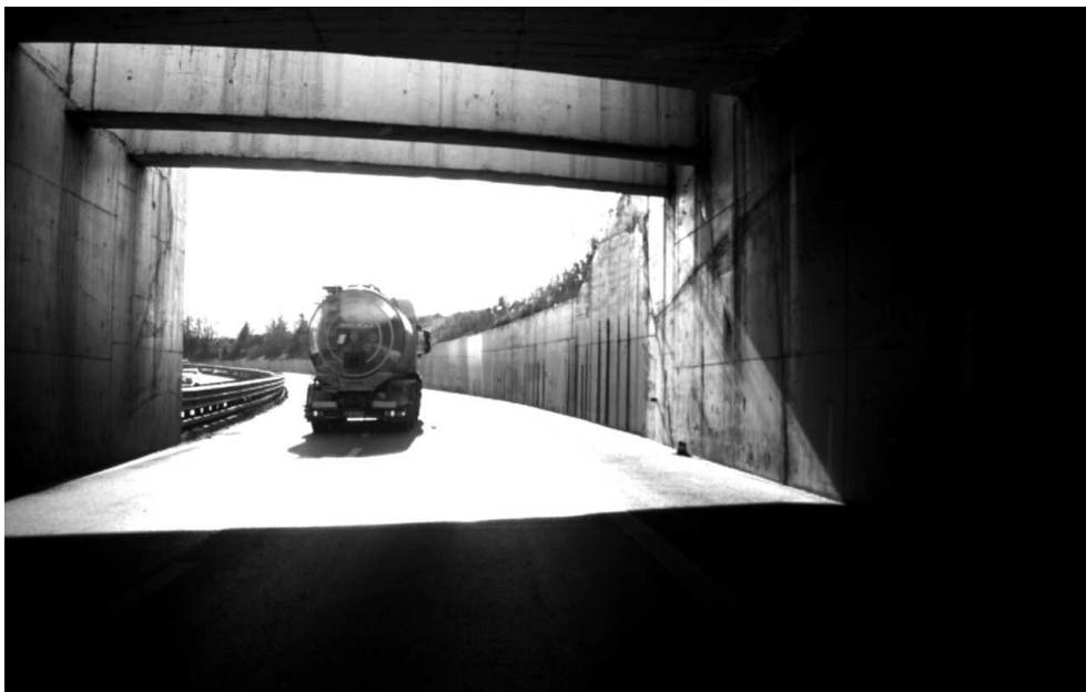
Figure 2.5: Sun's reflection can wipe the marks from the image.
