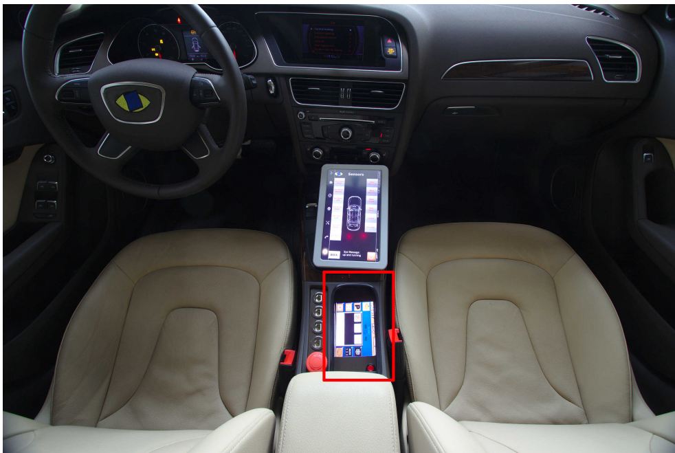
Figure 1.15: AEVIT control panel.
