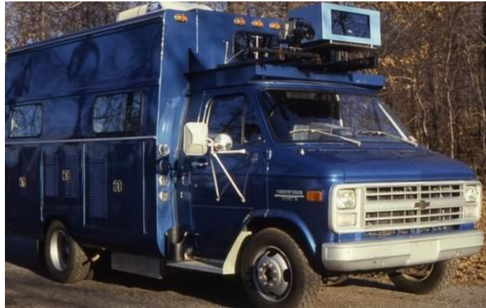
Figure 4: ALVINN autonomous vehicle, driven by a neural network.
