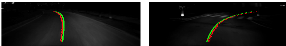
Figure 2.24: CenterNET in nighttime environment (red) with ground truth (green).
