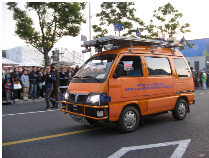
Figure 8: Porter: the electric vehicles that faced VIAC, equipped with solar panel for extended autonomy.
