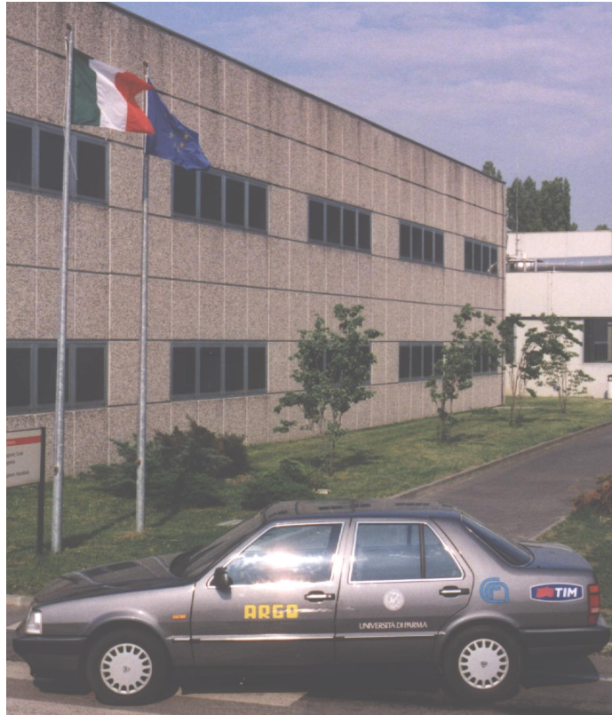
Figure 5: The ARGO car driven about 1900Km of highway with automated steering.
