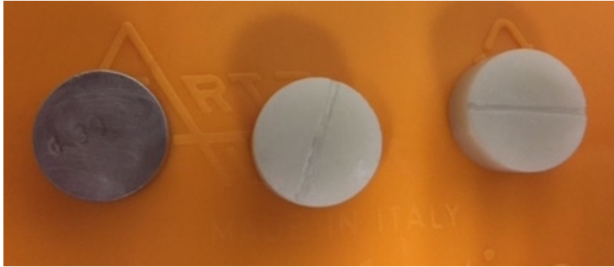
Fig. 5.1 - Samples used in the tests (center and right) and metal cylinder used to check the focus of the laser beam (left). Notice the groove for placing the FBG sensor in the centre of the sample surface.
