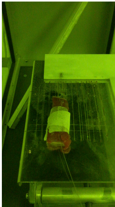
Fig. 4.3 - One of the samples during laser irradiation: it may be appreciated the optical fiber in the centre of the specimen.
