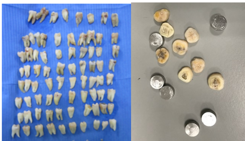
Fig. 6.1 - (left): the extracted human teeth used for the test; (right): sections obtained and steel cylinders used for laser focal distance adjustment.
