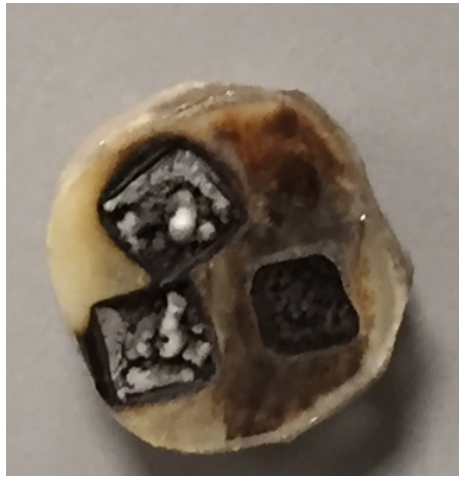
Fig. 6.2: Optical microscope observation sample irradiated with a peak power of 7.5 kW without air/water spray: a great amount of melting and carbonization can be appreciated.
