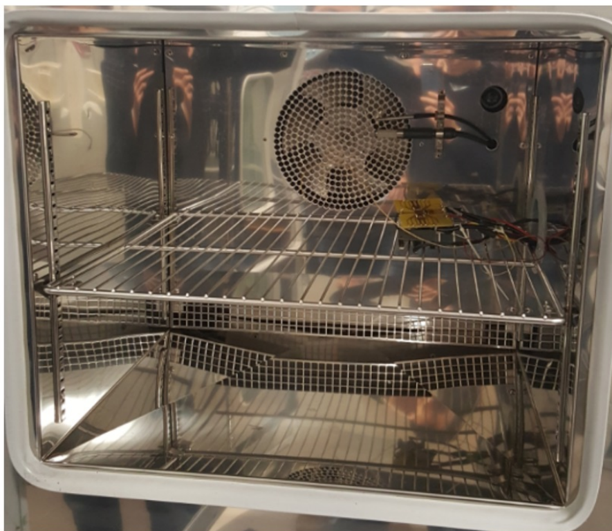
Figure 6.9: DUT in the climatic chamber.
