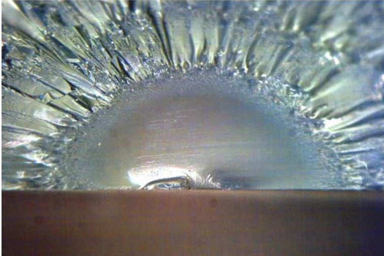
Figure 3.3: Fracture mirror of a plate broken under a four-point bending test [23].
