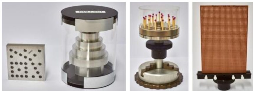
Figure 19: Mandatory reference standards inside the ISO test survey (left): PTB hole plate AI2 size 48 mm × 48 mm × 8 mm with 28 holes of 4 mm in diameter and NMIJ step cylinder SC1 with maximum outer diameter of 50 mm and central hole 8 mm in diameter inside PMM 19 .
