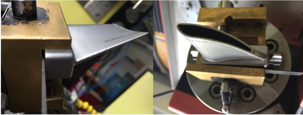
Figure 73: example of voluntarily positioning error, obtained by manually inserting a calibrated foil of 0.6mm into the turbine blade specimen fixturing system
