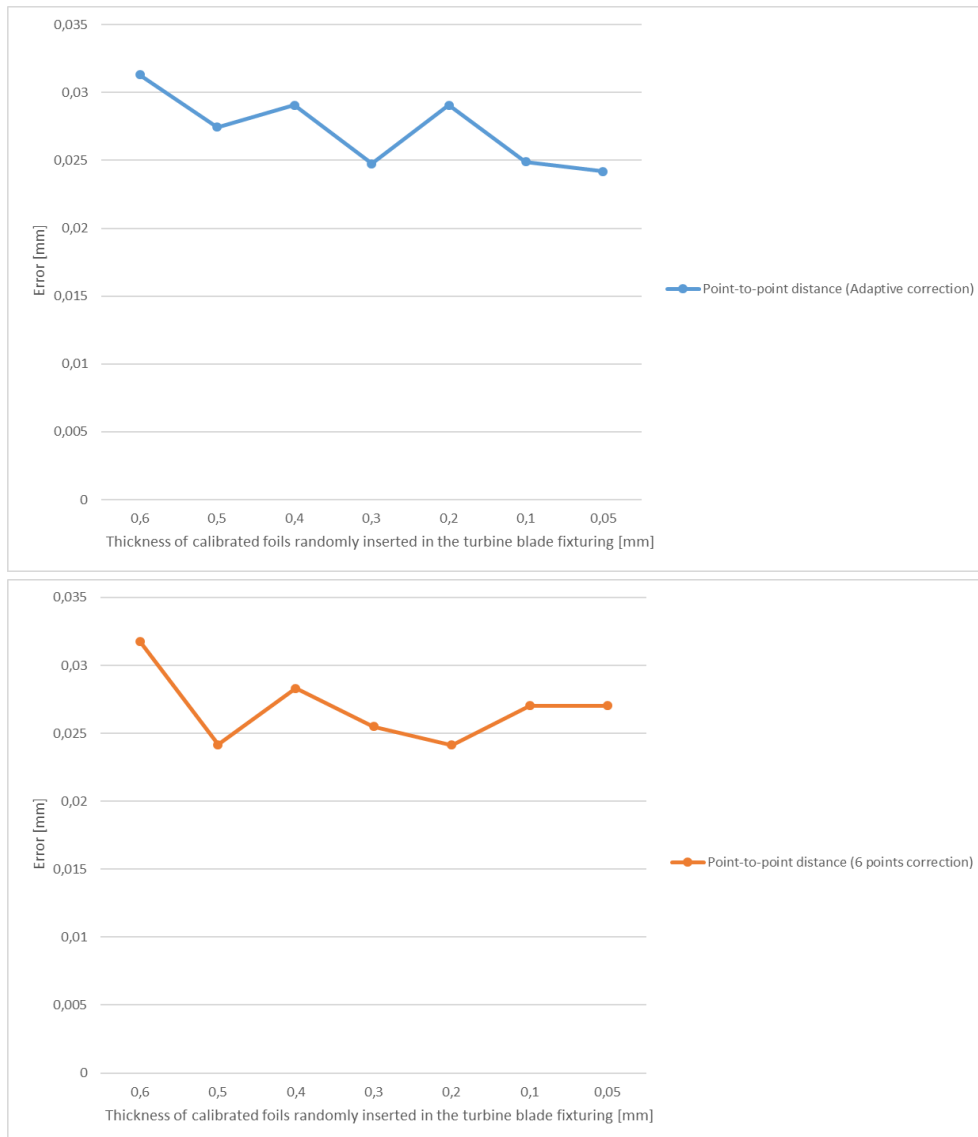
Figure 74: positioning procedures repeatability test; in blue the procedure repeated with the local adaptive positioning procedure, in orange the same test repeated with the six points constrained one
