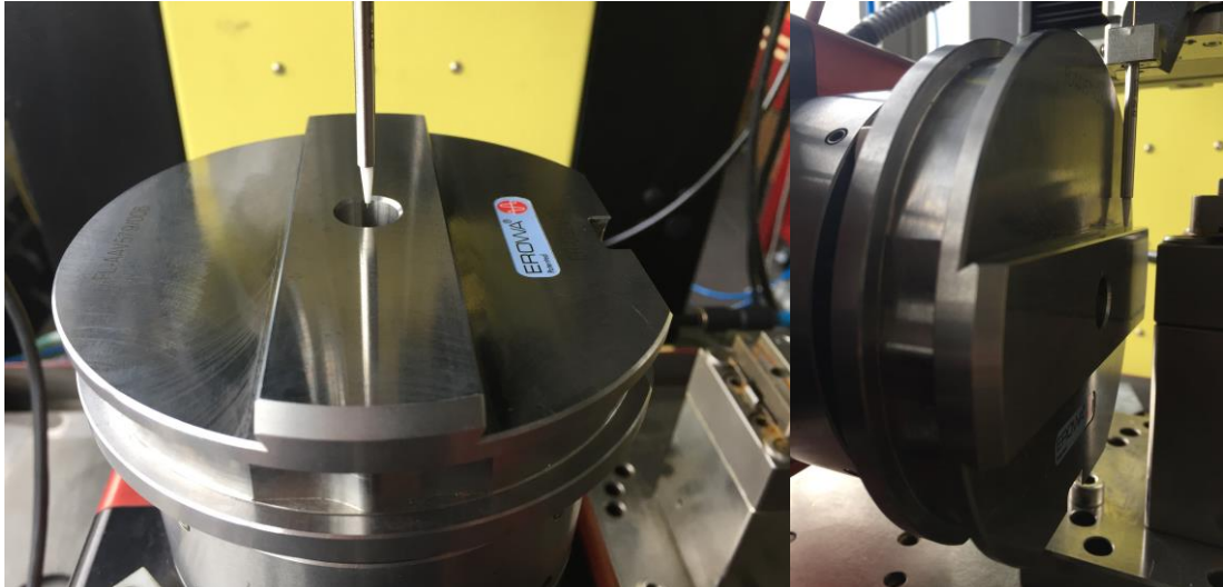
Figure 61: standard rotation centre (i.e. Point C) localization procedure, via touch probing
