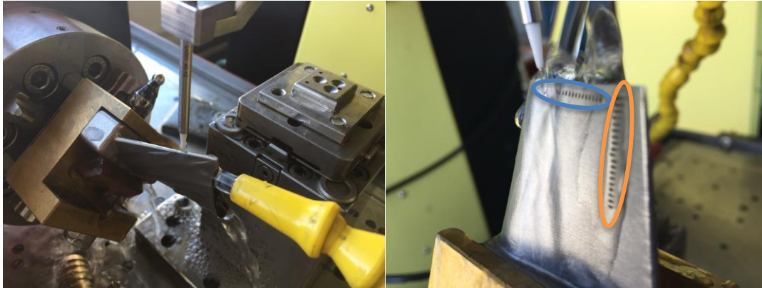
Figure 71: turbine blade specimen micro-EDM machining operations after positioning procedure has been implemented
