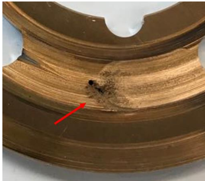
Figure 4-13: Photograph of the tested port plate damaged by cavitation, fault 2.
