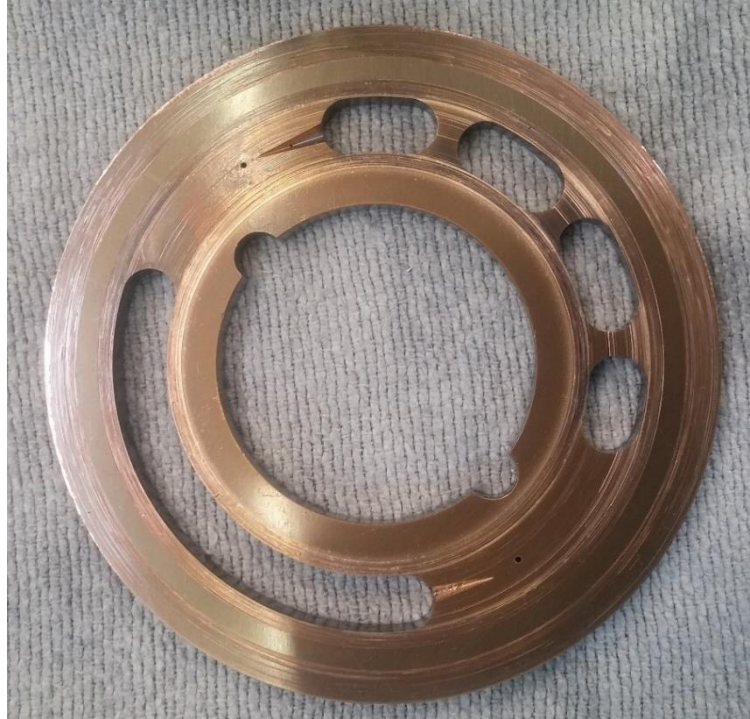
Figure 3-7: Worn port plate.
