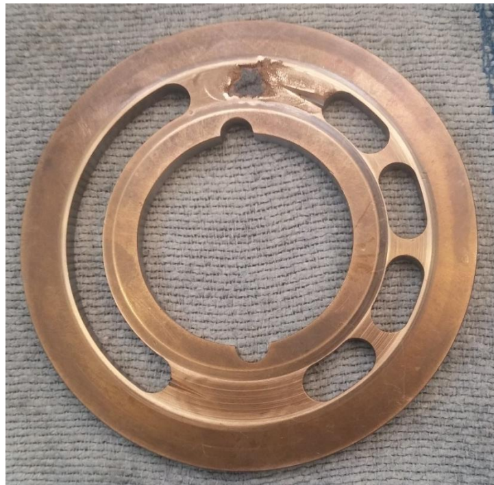
Figure 3-8: Port plate with cavitation erosion.
