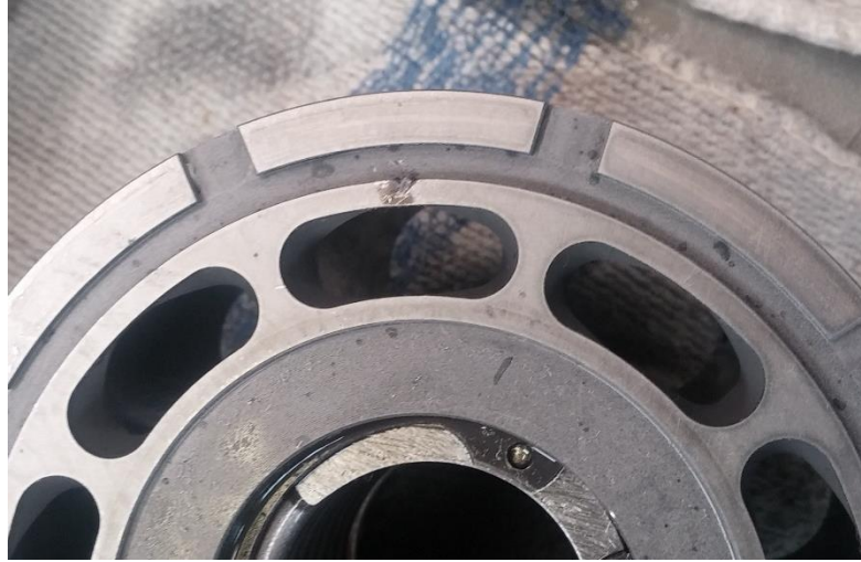
Figure 3-13: Artificially damaged piston block.
