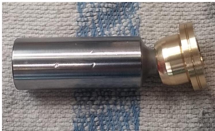
Figure 3-12: Artificially damaged piston.
