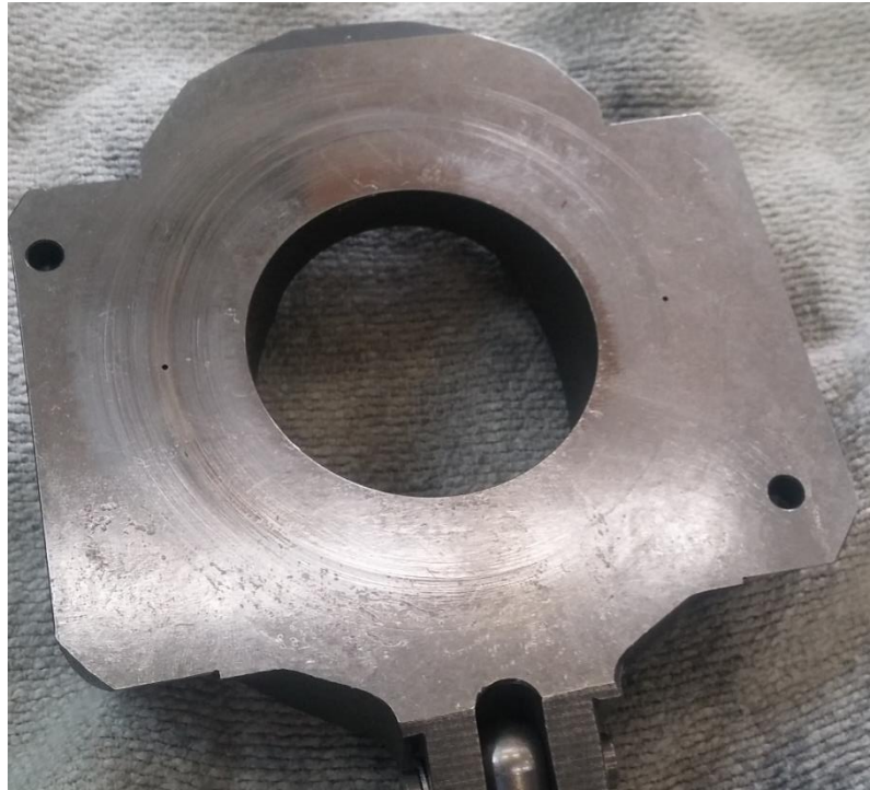
Figure 3-9: Worn swash plate.
