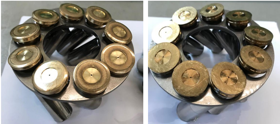
Figure 4-12: Photograph of the tested worn slippers (left), fault1, along with the slippers of the flawless pump (right).
